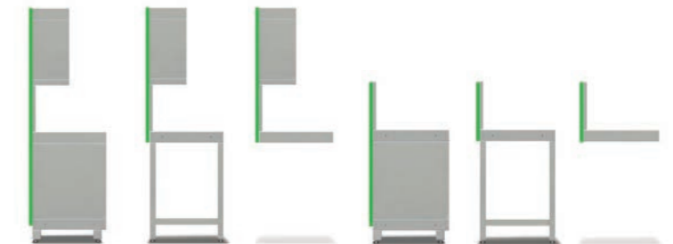
BK001 To connect: Wall cabinet Back Panel Base Cabinet BK003 To connect: Wall cabinet Back Panel Workbench BK003 To connect: Wall cabinet Back panel Bridging Unit BK004 To connect: Back Panel Base Cabinet BK005 To connect: Back Panel Workbench BK005 To connect: Back Panel Bridging Unit
