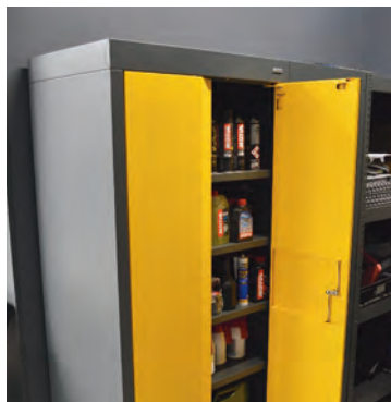
Store with COSHH cabinet
